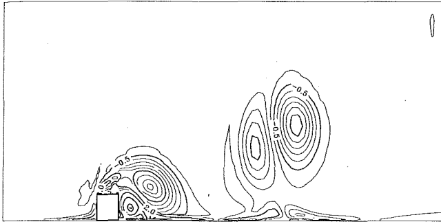
Fig. 10 Case 3: Flow past a rib on a sliding wall. Instantaneous vorticity contours for the unsteady flow case, Re = 500
